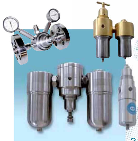
COMPRESSED AIR UNITS 316 L Material brass, stainless steel 316 L Ports in body from 1/4" to 4" and flange Working pressure 30/50 bar to 200 bar
